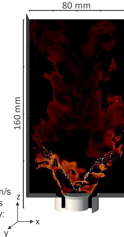
Schematic of the burner geometry Instantaneous soot volume fraction and liquid phase measurement
